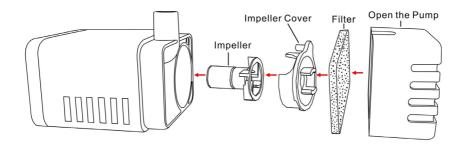
If after some time the pump starts losing power or stops working you should check for the build up of sediment or scale in the filter or in the pump housing. The filter housing can be removed by pressing down on the bottom of the filter housing. Clean with fresh water.
