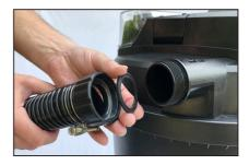
**Step 9 -** Now refit all the hoses again — remember to insert the flat gaskets and tighten the locking nuts.
