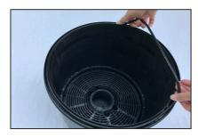
Step 8 - Fit the O-ring in place on the top of the cannister (to facilitate the placement of the lid, you can use silicone grease (preferred) or make the O-ring wet. The lid can then be pressed in place and the large clamp be mounted from the hinge side and locked.
