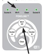
Press and hold Wi-Fi button for 5 sec. until LED is flashing fast.
