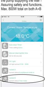
28. Socket B can be used for all pond-equipment like feeder, dosage pump, light etc. Max, 800W total on both A+B
